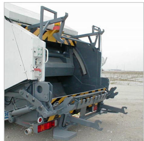
Zenith BLT100 with trunion arm - suitable for 120 to 1,100 ltr DIN bins
