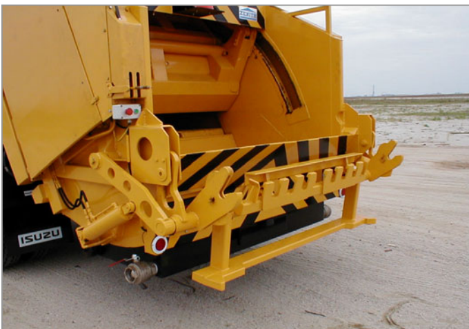
Zenith BLT100 w/o trunion arm - suitable for 120 to 1,000 ltr DIN bins
