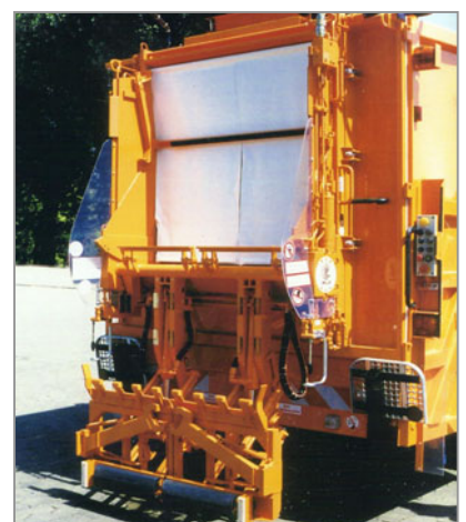
Zoeller 300 - Divided comb bin-lifter for 80 to 1,300 ltr DIN bins
