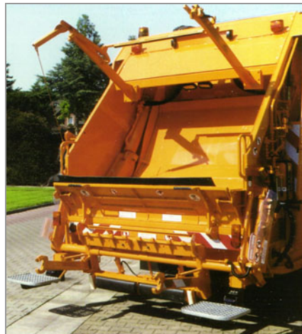
Zoeller 249 - Open hopper comb lifter for 80 to 1,300 ltr DIN bins
