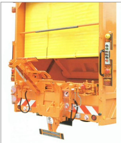
Zoeller 202 - Low level divided bin-lifter for 80 to 1,100 ltr DIN bins
