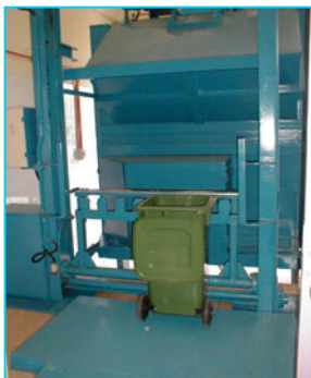
Binlifter designed to lift 2 X 240 ltr OR 1 X 660 ltr DIN bins.
