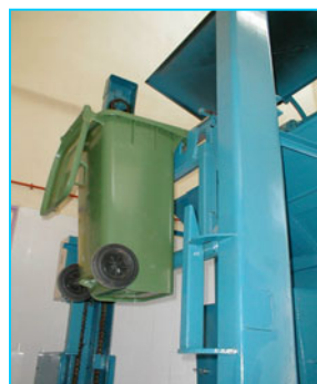
Binlifter designed to lift 2 X 240 ltr OR 1 X 660 ltr DIN bins.
