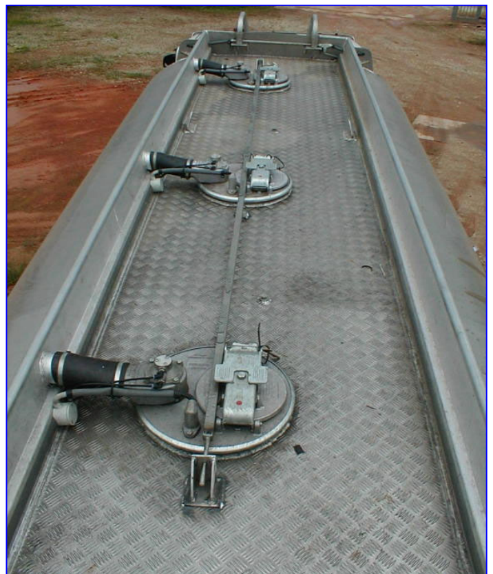
1,000mm wide FLAT cat-walk Concealed wiring & hoses in the continuous-extruded coaming All components are lower than roll-over coaming
