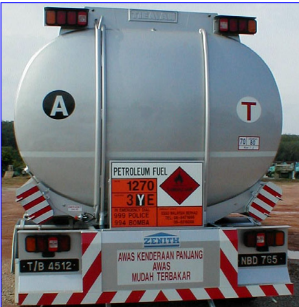
Semi-elliptical maximises the cross section, lowered center of gravity, increases volume & shorter barrel length .
