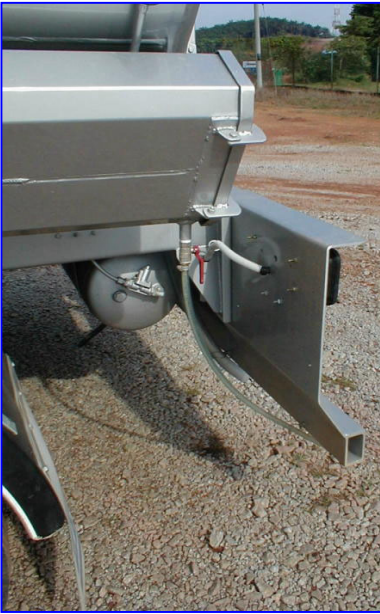
Drain-off for hose box
