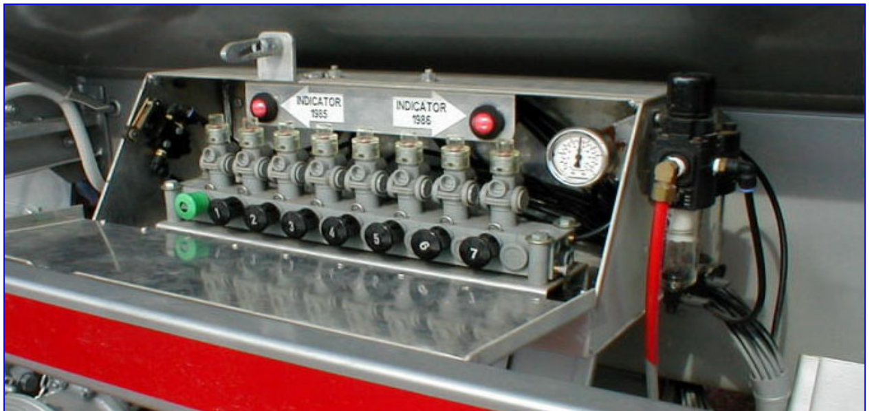
Lockable Control box fitted with auto-cut off roller-valve. Air system independent of all other services.
