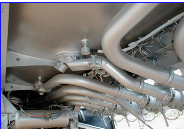
Continuous piping (without weld joint) reduces risk of cracks.
