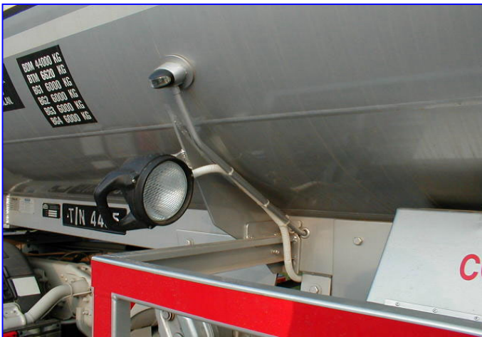
vapour-proof work lamp & durable LED side-markers and aluminium conduit reduces damage of wires cause by stones & gravels .
