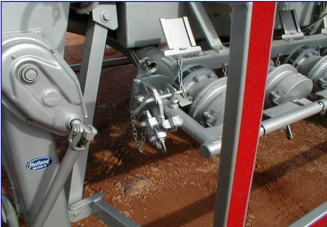
Air-interlock valve shuts off the systems when the lock-bar is not lifted. Design of lock-bar prevents latch-release and rotation of dust-caps and operation of API levers.
