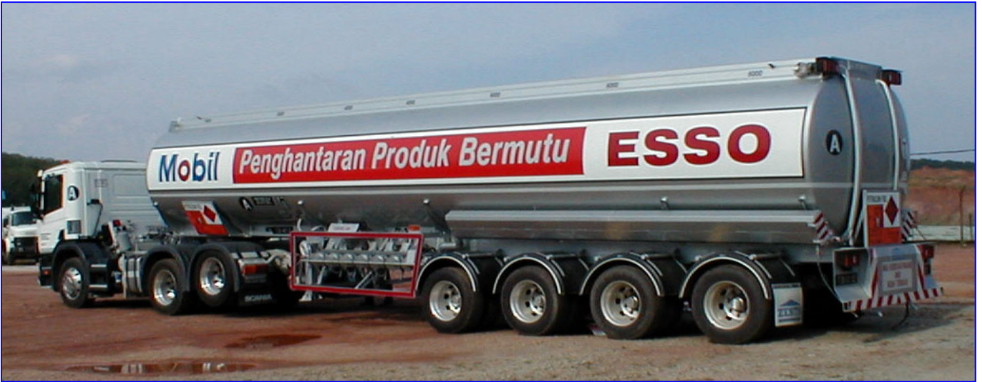
Picture shows a 7 compartment , 40,000 ltr (39,000ltr safe fill capacity) on quad-axles with full ABS , aluminium hub & rim. Tank Length = 11.83 m , Overall Height 3,520 +/- 50 mm Tare weight 6,800kg (+/- 3%) .Delivered to Esso June 2001.
