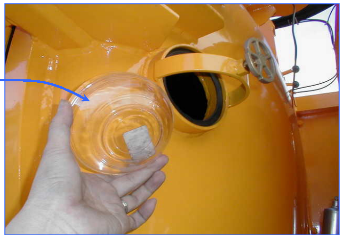
Sight glasses can be dismantled in less than 15 secs for cleaning and maintenance and re-installed in just as quick a time .
