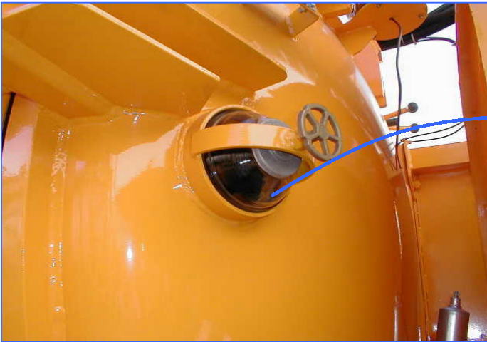
Sight glasses can be dismantled in less than 15 secs for cleaning and maintenance and re-installed in just as quick a time .
