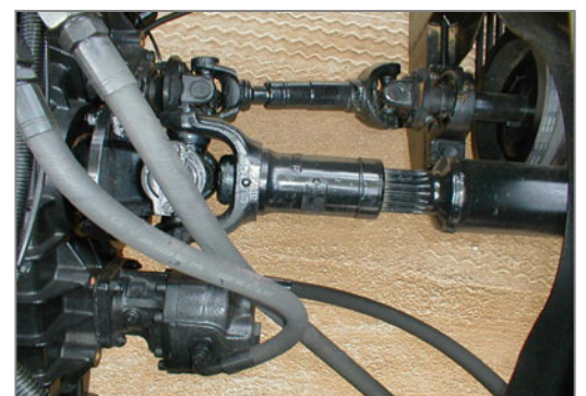
Driven by Split-shaft PTO a) vacuum pump via pulley b) hydraulic pump via direct drive
