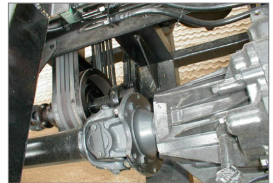
Pneumatic operated throttling to bring the pump to the required rotor speed.
