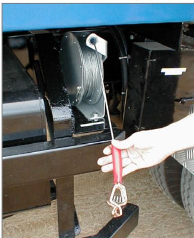
Earthing Strap (mandatory for refinery operation)
